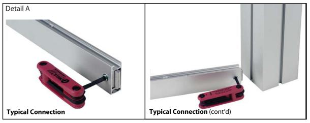
Most horizontal extrusion connections have a patented expandable lock. This lock inserts into the groove of an opposing extrusion. Tightening the lock with the Hex Key Tool expands the lock and creates a strong positive connection.
